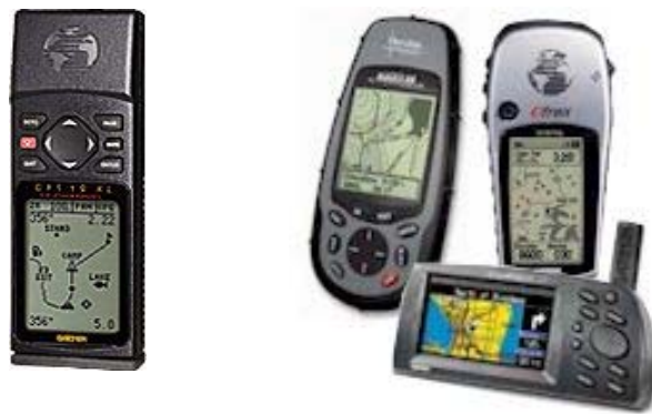
Gambar 12 : Receiver GPS Tipe Navigasi
