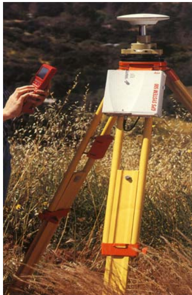
Gambar 13 : Receiver GPS Tipe Geodetik
